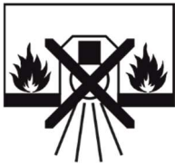
Suitable for fastening on non-flammable surfaces only
