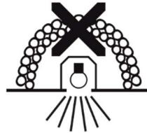
Unsuitable for covering by heat insulation material
