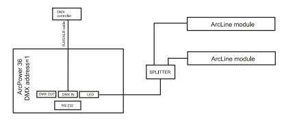
ArcLine units are supplied with 1.5 m of cable for direct connection to the ArcPower drivers.
