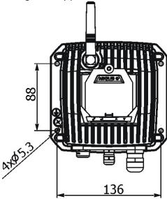
Four holes with diameter of 5.3mm in the control unit are intended for mounting on a flat, non-flammable surface. The length of the connection cable between the ArcPower 24 Outdoor and the LED unit should not exceed 20 m (at 700mA load) or 80m (at 350mA load).
