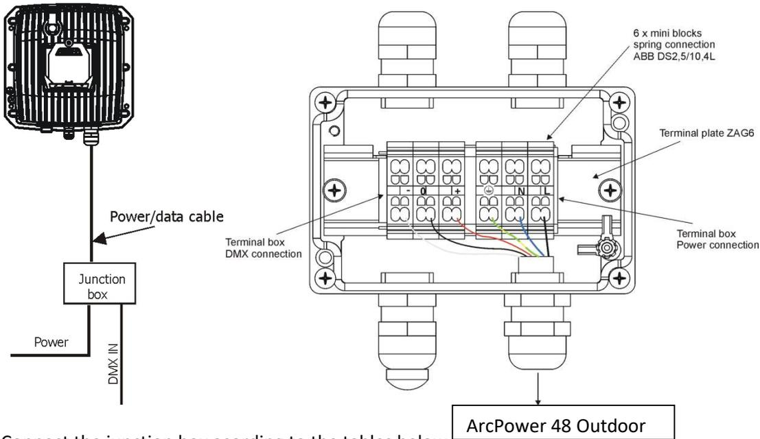
Connect the junction box according to the tables below
