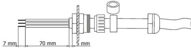
**4 x Reducing seal** (P/N 13051388) - enclosed, standard seal
