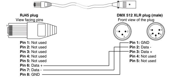
**2.**RJ45 patch cables category 5 that connect the ArcPower SmartWhite 72 each other are wired 1:1,that is,pins with the same numbers are connected together.
