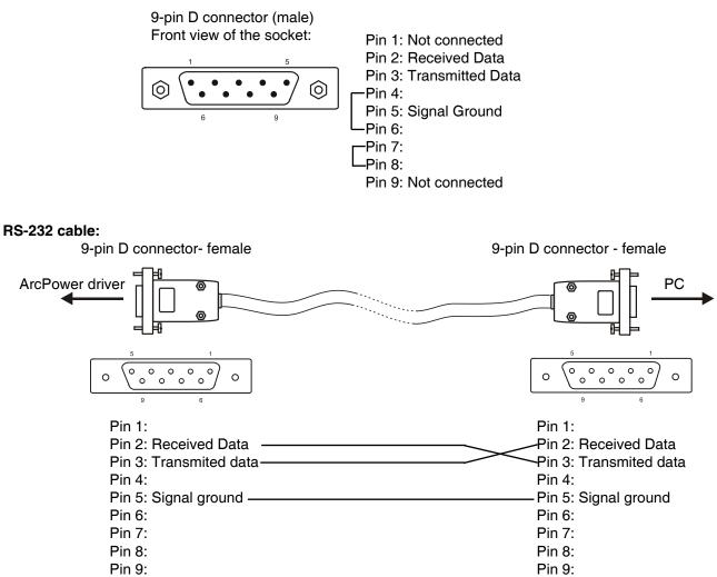
The maximum cable length according to the standard is 15 metres or the cable length equals to a capacitance of 2500 pF.
