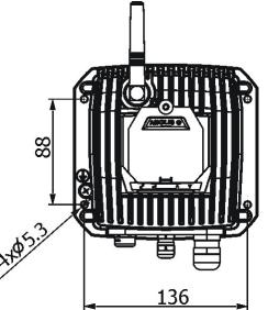
Four holes with diameter of 5.3mm in the control unit are intended for mounting on a flat, non-flammable surface. The length of the connection cable between the ArcPower 24 Outdoor and the LED unit should not exceed 20 m (at 700mA load) or 80m (at 350mA load).
