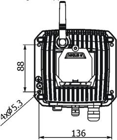
Four holes with diameter of 5.3mm in the control unit are intended for mounting on a flat, non-flammable surface. The length of the connection cable between the ArcPower 24 Outdoor US and the LED unit should not exceed 20 m (at 700mA load) or 80m (at 350mA load).
