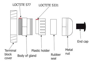
The cable gland M20 MS with a standard seal serves for a cable of diameter of 6-12mm, for smaller diameter of cable (4-8mm) you have to remove the original seal from the cable gland M20 and use the enclosed reducing seal instead of it. The reducing seal for diameter of cable 4-8mm (P/N 13051388) is enclosed in the Booster box.
