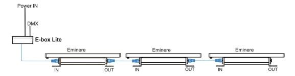
Number of connected Emineres to one E-box output depends on a cable length, power voltage, type of Eminere and E-box and operation mode.
