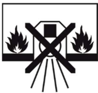
Suitable for fastening on non-flammable surfaces only
