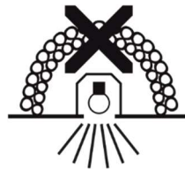
Unsuitable for covering by heat insulation material
