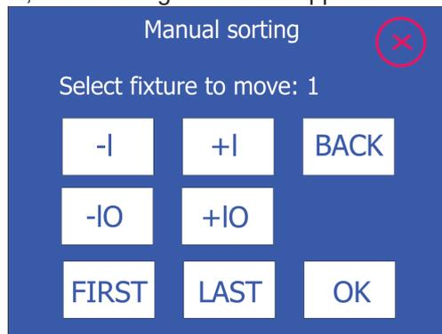
2. Select desired fixture by means of -1 and +1 buttons (movement by 1 position) or -10 and +10 buttons (movement by 10 positions) or FIRST and LAST buttons (movement on first/last fixture). Selected fixture will light in red colour.
