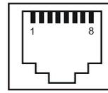
**Pin 1:** TX+                      **Pin 5:** Not connected
