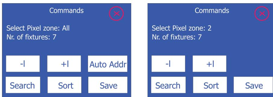
**Search Pix** - this function checks all pixel modules connected to the ArcPower Unit Pixel.
