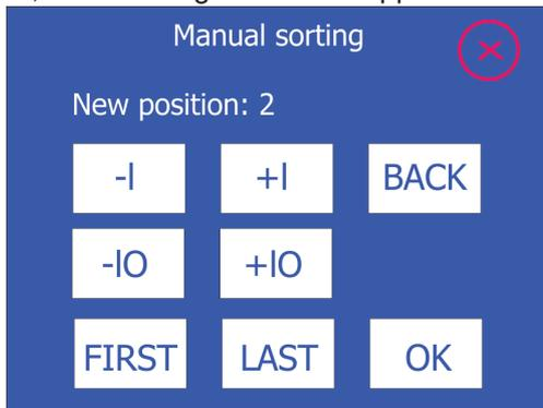
3. Select new position of the fixture by means of -1 and +1 buttons (movement by 1 position) or -10 and +10 buttons (movement by 10 positions) or FIRST and LAST buttons (movement on first/last fixture). Fixture will light in green colour.
