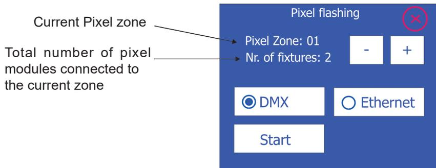
2. By means of the   buttons select zone at which you need to upgrade pixel modules (information about pixel modules is available in the menu Information-->Zone Info).
