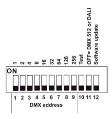
DIP 10 - if switched to ON=test light (the fixture lights at 3200K (RGBW, TD version))
