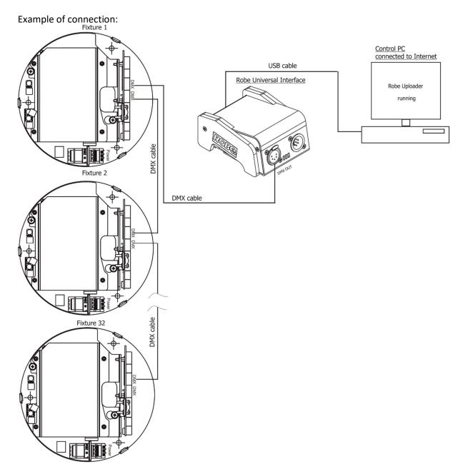
The fixtures has to be connected in a daisy-chain (max. 32 fixtures) and via the Robe Universal Interface/Robe Universal Interface WTX and a USB cable connected to the control PC with the Robe Uploader running. The fixtures have to be connected to power. The control PC should be connected to the Internet.
