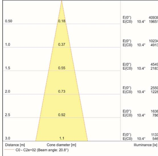
Fixture set at 3200K, secondary power (emergency operation), 20° beam angle
