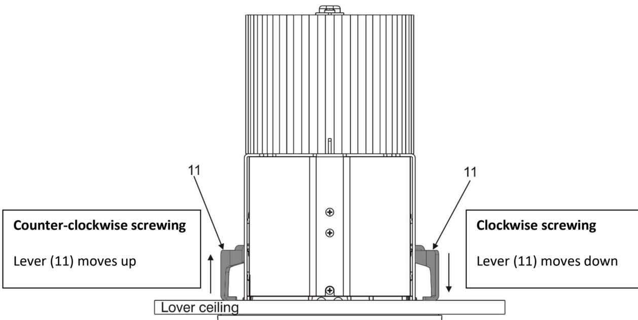
10. Insert the frame with reflector (3) to the Ambiane HP111 housing (4) and push and turn it clockwise until it snaps into locks (2) in the Ambiane HP111 housing (4).
