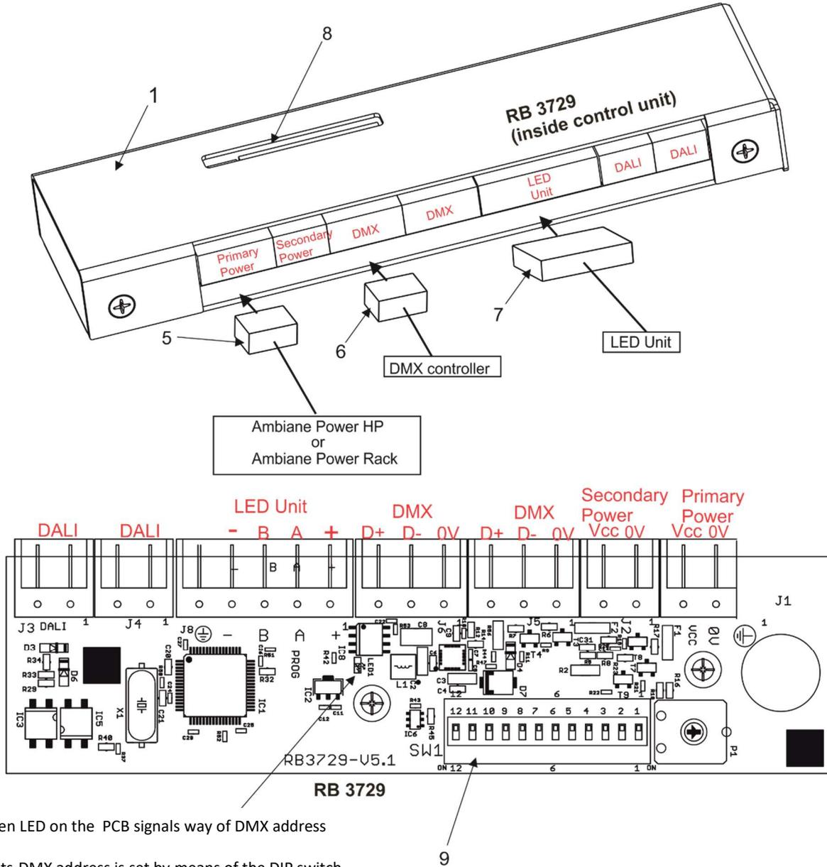
The green LED on the PCB signals way of DMX address setting:
