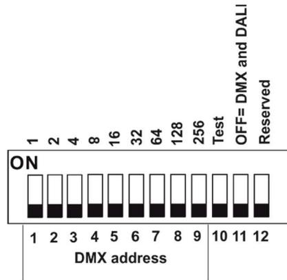
DIP 10 - if it is switched to ON=test light (the fixture lights at 3200K (for RGBW and TW version))
