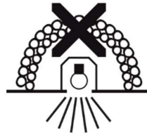
Unsuitable for covering by heat insulation material
