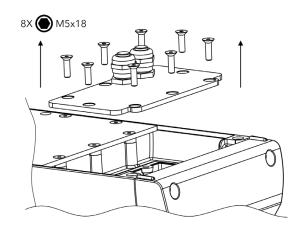
Uncover junction box located on the bottom side of luminaire.
