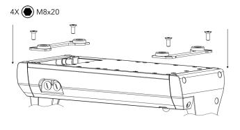
Mount pair of rubber feet using 4 screws.
