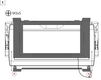
Unscrew two screws and split accessory to two parts. Place each part onto the luminaire's head and screw them together.
