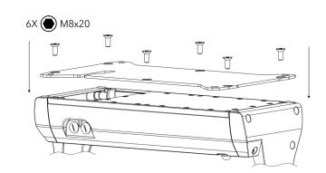
Mount the adaptor using 6 mounting screws.
