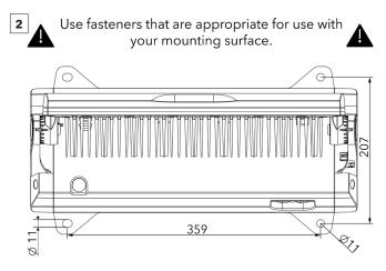
Drill holes to the surface according to holes spacing. Mount Divine via mounting holes on the surface.
