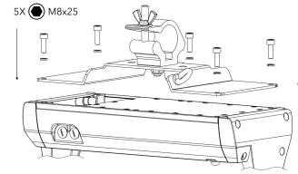
Mount the adaptor using 5 screws.
