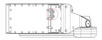
Inlets for power and data from bottom side of the luminaire.
