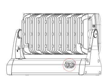
Inlets for power and data from side of the luminaire.
