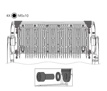
Secure accessory by 4 screws with spring washer at the back side of luminaire's head.
