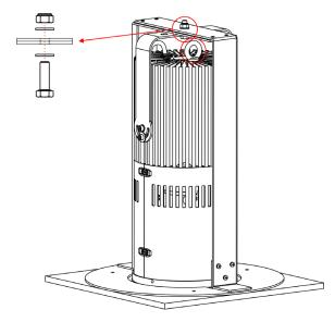
Fasten yoke of Ambiane XP56 to the adaptor with screw, nut and washers provided with adaptor.
