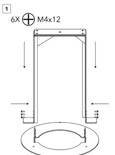
Assemble installation tool and secure it by six screws.
