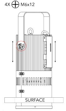
Adjust the fixture into desired position and tighten all loosened screws.
