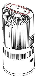
Drill holes in upper ceiling (or other construction) according to mounting holes on the Yoke.
