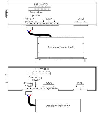
Install terminal block on Primary power cable leading from Ambiane Power Rack or Ambiane Power XP and connect it to the Control Unit.
