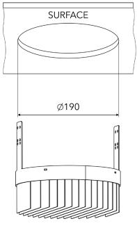
Without using a Trim or a Louver, prepare opening of 186mm diameter in lower ceiling.
