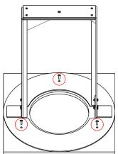
Mount installation tool on the surface and fix by three screws.
