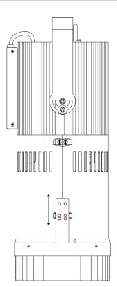
There are three sets of mounting holes on the Louvre. (Size of the luminare depends on type of used optic) When the Louver is mounted on luminaire, one of those sets will match mounting holes on housing of the luminaire.
