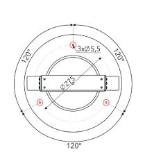
Prepare holes in the surface (lower ceiling) according to spacing of mounting holes on base plate.
