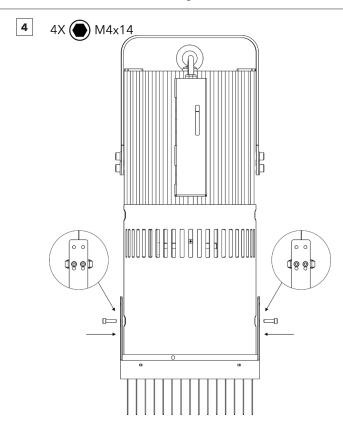
Secure the Louver by means of two M4x14 (enclosed with the Louver) on each side of the Ambiane XP56's housing.
