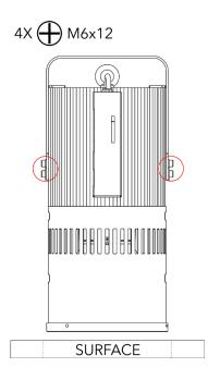
To move the Yoke/luminaire up or down loosen both screws on each side of the Yoke.
