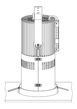
Lift up both Spring Clips and slide the Trim onto the housing of the Ambiane XP56 through the opening in the lower ceiling.
