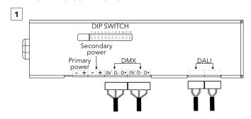
Install terminal blocks on DMX or DALI cables and connect them to the Control Unit.
