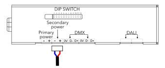
Install terminal block on Secondary power cable and connect it to the Control Unit.
