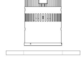
Fasten the luminaire to the surface with suitable fasteners. Secure the Ambiane XP56 to the ceiling (construction) via a safety wire pulled through the mounting lug (highlighted on picture above)
