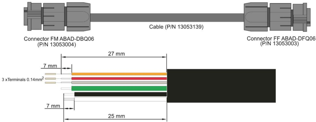
3. Put parts of the connector on the cable (5) and connect wires to the connector. First connect power wires (L,N, Earth) and after that data wires (D+, D-, 0V). Avoid excessive torsion of data wires!
