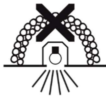
Unsuitable for covering by heat insulation material
