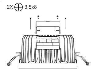
Unscrew 2 screws on the control unit and remove plastic co-
