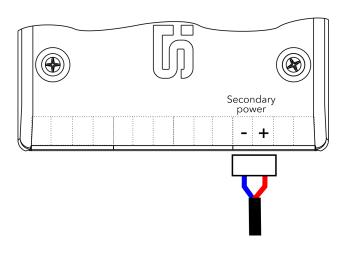
Install terminal block on power cable for secondary power and connect it to the Secondary power connection of Ambiane AP's control unit.
