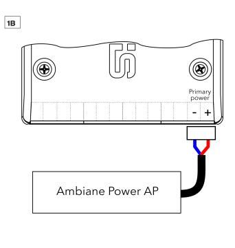
Install terminal block on power cable (from Ambiane Power Rack or Ambiane Power AP) and connect it to the Primary power connection of Ambiane AP's control unit.
