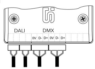
Install terminal blocks on DMX or DALI cables and connect them to the control unit.
