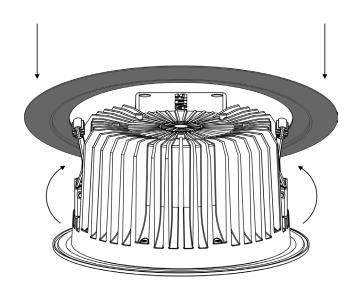
Slide Adapter ring under the control unit and above both spring clips.
