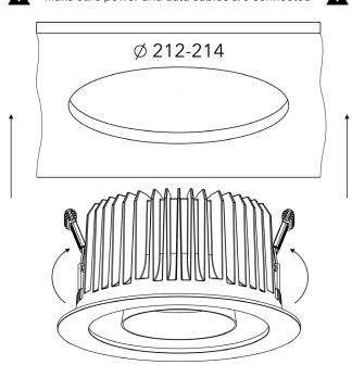
Lift up spring clips on both sides, insert luminaire into ceiling opening and release spring clips to hold lumaire in place.
