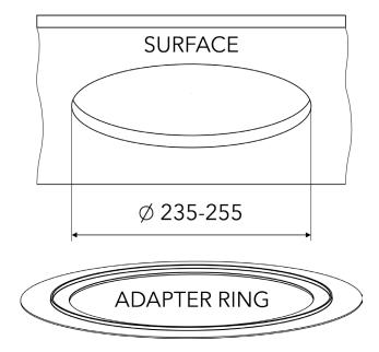
Use of the Adapter ring is recommended in case of a bigger ceiling opening. See step 6.B before connecting power and data cables.
