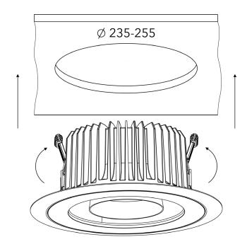
Adapter ring installed on the luminaire.
