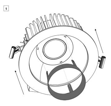
Insert the Anti-Glare ring into the Ambiane AP's reflector until
