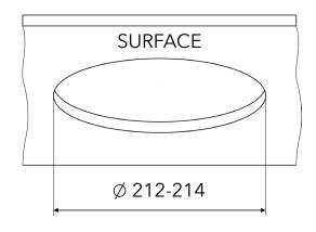
Prepare mounting hole with diameter between 212-214 mm.
