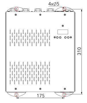
Fasten the ArcPixel Power to surface via four mounting holes and four screws.
