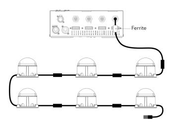
ArcDot line may be done with in/out connection or by using T-connectors (1 ArcDot can be connected to T-connector). Max. number of ArcDots per output is 35. Max. cable length of 1 LED output is 65m at 35 ArcDots and 100m at 25 ArcDots per LED output.
