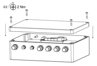
Install top cover making sure the gasket is in good condition and is positioned properly in the groove. Before applying the torque, make sure the thread is clean and functional.
