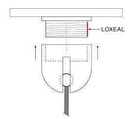
Screw the Spherical Cap (with the Hanging Wire) to the Ceiling Plate. Use of thread glue LOXEAL 5503 is recommended.
