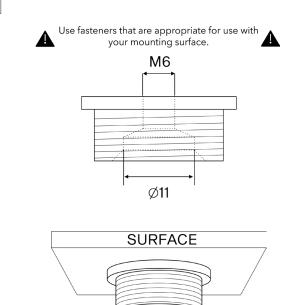
Fasten the Ceiling Plate M6i to the lower ceiling with suitable fastener.
