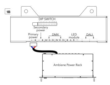
Install terminal block to power cable (from Ambiane Power Rack or Ambiane Power HP) and connect it to Primary power socket of the control unit.
