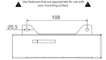
Fasten the control unit on the ceiling by means of two holes in the control units housing.
