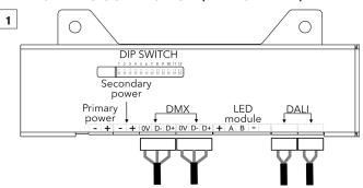
Install terminal blocks on DMX or DALI cables and connect them to the control unit.
