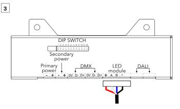
Pull the LED unit's cable through prepared hole in the ceiling and secure it above ceiling. Install a terminal block on the cable and connect it to the control unit.
