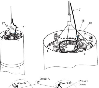
Length of the LED unit supply cable (7) should be adequate, it is not suitable to make "loops" of cable on the LED unit heatsink. Max. one "loop" can be created.
