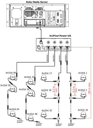
The minimum cable length of 0.3m between two T-connectors has to be kept in case that the pixel sorting is executed manually from the ArcPixel Power-US menu.
