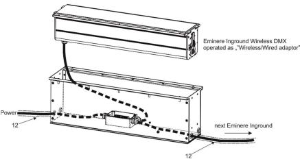
The supply cable to the mounting sleeve and power/data cable from the mounting sleeve must be placed in a protective tube (12).
