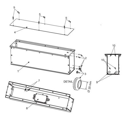
5. Connect the Eminere Inground (13) and all needed cables to the junction box (8).
