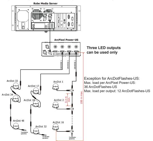
Every ArcDot line has to be terminated with the passive terminator!
