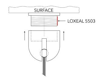
Screw the Spherical Cap (with the Hanging Wire) to the Ceiling Plate. Use of thread glue LOXEAL 5503 is recommended.
