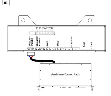
Install terminal block to power cable (from Ambiane Power Rack or Ambiane Power XP) and connect it to Primary power socket of the control unit.
