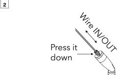
Press down pins on the hanging wires anchors for length and downward orientation adjustment.
