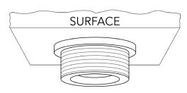
Fasten the Ceiling Plate M6i to the lower ceiling with suitable fastener.
