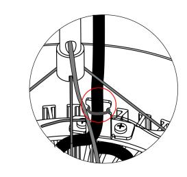
Fasten the LED unit's cable to holder using a cable binder.
