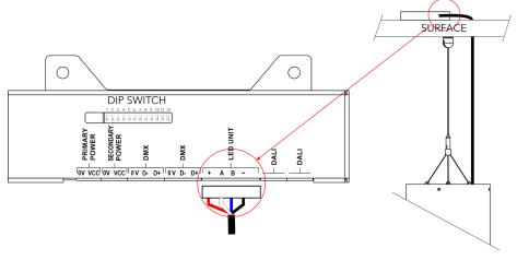
Pull the LED unit's cable through prepared hole in the ceiling and secure it above ceiling. Install a terminal block on the cable and connect it to the control unit.
