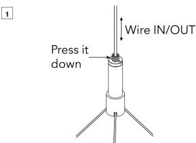
Press down the pin on the wires connector for length adjustment.
