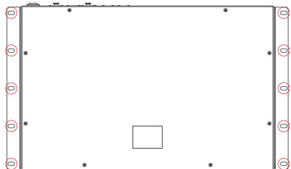
Drill holes to the surface according to holes spacing. Mount ArcPower Unit Pixel via mounting holes on the surface.
