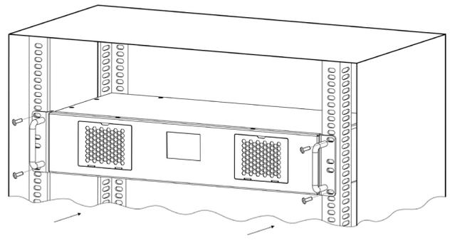
Fasten the ArcPower Rack Unit into rack by means of two screws on each side of the Ambiane Power Rack .
