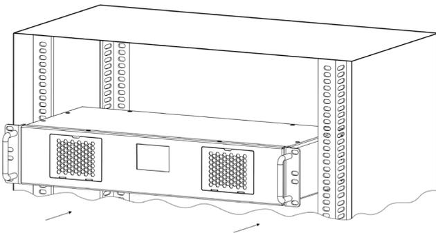
Install ArcPower Rack Unit into the rack case.
