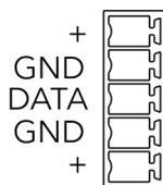
5-PIN for terminal block connection
