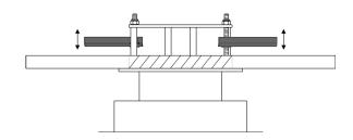
Insert the fixture into the ceiling mounting hole.
