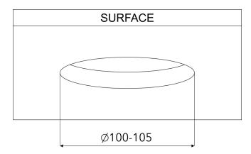
Standard mounting hole with diameter of 100-105mm.
