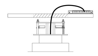
LED unit connected to control unit prior to mounting.
