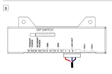
Install terminal block on LED unit's cable and connect it to the control unit.
