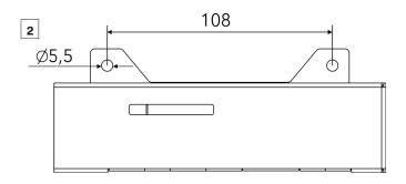
Place control unit above the ceiling through the ceiling opening.
