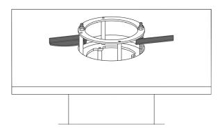
Tighten the holders on both sides until the fixture is firmly secured to the ceiling.
