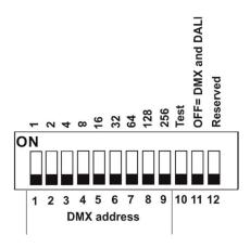
DIP 10 - if it is switched to ON=test light (the fixture lights at 3200K (for RGBW and TW version))
