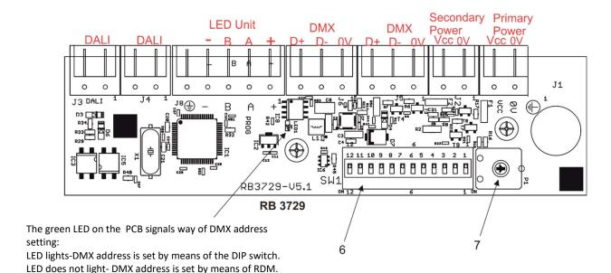
Note: The trimmer (7) allows you to set a light intensity (for secondary power only). This trimmer is accessible by aperture (5) in the cover of the control unit (1).
