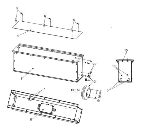
Connect the Eminere Inground (13) and all needed cables to the junction box (8).
