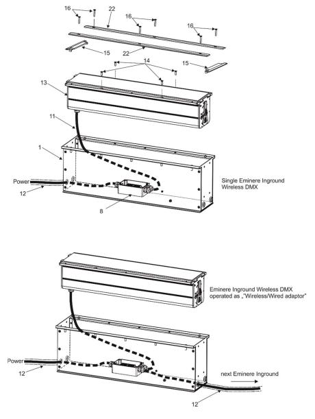
The supply cable to the mounting sleeve and power/data cable from the mounting sleeve must be placed in a protective tube (12).
