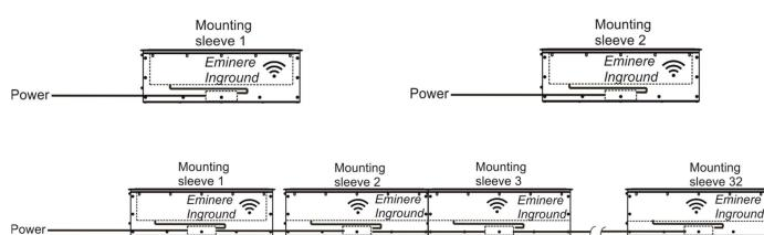
The Eminere Inground can be only linked to a transmitter by running the link procedure at DMX transmitter .
