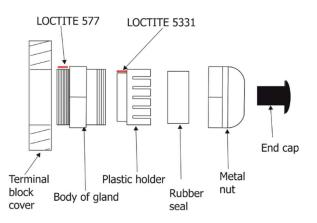
We recommend to apply an adequate layer of the paste LOCTITE 5331 on the plastic holder of the cable gland before inserting it into the body of the gland and an adequate layer of the paste LOCTITE 577 on the thread of the gland body in case that you need to unscrew and remove the cable gland from the housing of the junction box and and screw it back to the housing.
