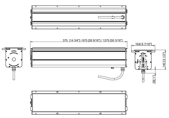
**Dimensions with mounting sleeve (**All dimensions in mm [inch])
