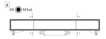
Fasten the adaptor to the fixture with 4 screws.
