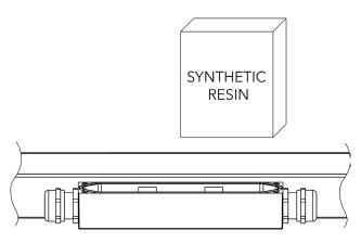
After checking all connections, fill the connection box with synthetic resin. Make sure the end cap is inserted in any unused cable glands, and the earth ground wire is pulled from the junction box before filling it with resin. Read and follow all instructions stated on the resin bag prior to filling the junction box. The connection box has to be fully filled by resin.
