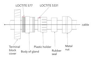
Apply Loctite 5331 thread sealant on the plastic holder and Loctite 577 thread locking compound on the gland body in the indicated locations prior to assembly.
