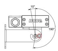
Loosen locking screws on both sides, adjust fixture to desired position and tighten locking screws on both sides.
