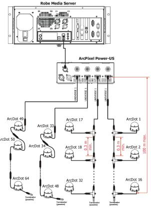
The minimum cable length of 0.3m between two T-connectors has to be kept in case that the pixel sorting is executed manually from the ArcPixel Power-US menu.
