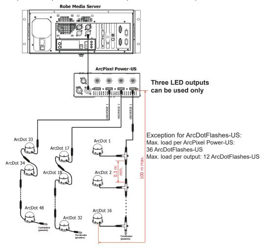
Every ArcDot line has to be terminated with the passive terminator!
