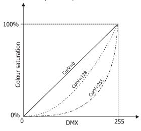
**RGBW 4ch Mode** - This function activates four channels RGBW mode (see DMX protocol) - for RGBW modules only.
