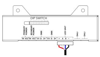
Pull the cable through the hole. Install terminal block on LED unit's cable and connect it to the control unit.
