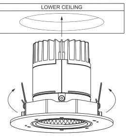
Lift up spring clips on both sides. Insert luminaire into ceiling
