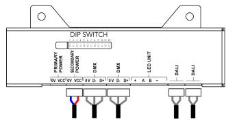
Install terminal blocks on SECONDARY POWER and DATA cables and connect them to the control unit.
