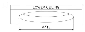
Prepare mounting hole with diameter of 115mm.
