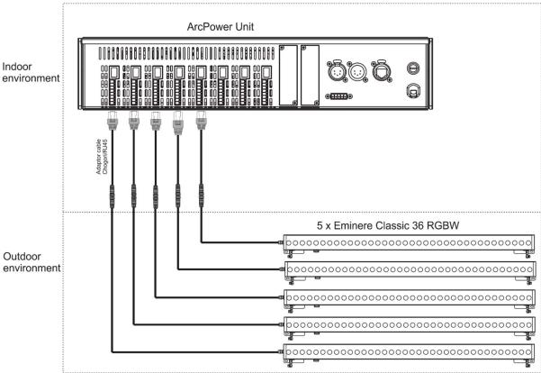
Fixture's Chogori connector is water protected according to IP 67 by mating with related Chogori connector. It cannot stay disconnected outdoor without covering the waterproof cap (optional item).
