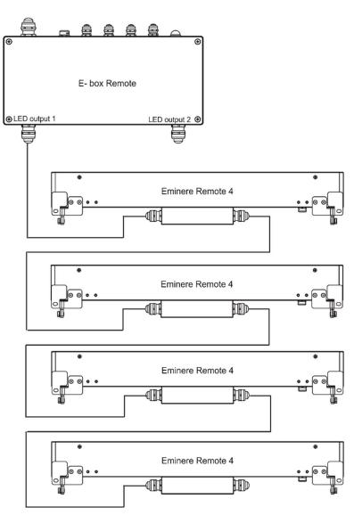
The table below states max. number of Eminere Remote modules connected to the E-box Remote/E-box Remote Basic.
