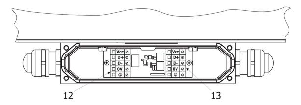
Wiring of connection blocks (12,13) in the junction box.
