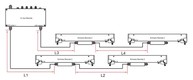
Max. number of Eminere Remote modules connected to the one output of the E-box Remote/E-box Remote Basic is stated in the following table.
