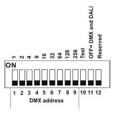
DIP 10 - if it is switched to ON=test light (the fixture lights at 3200K (for RGBW and TW version)) DIP 11 - has to be switched to OFF position to receive DMX 512 and DALI, position ON=0-10V control
