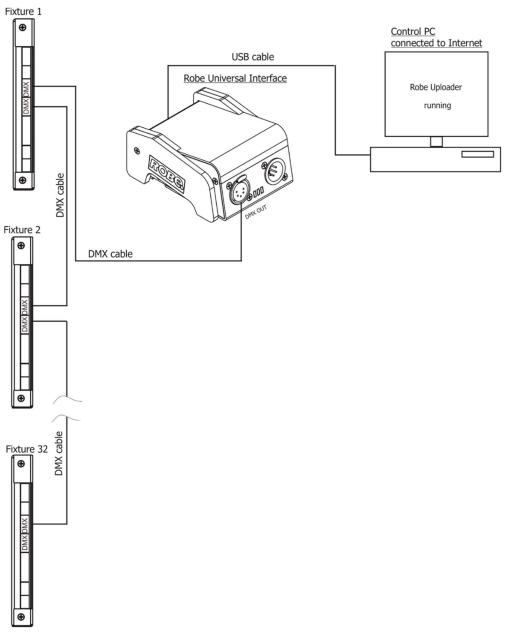
The fixtures have to be connected in a daisy-chain (max. 32 fixtures) and via the Robe Universal Interface/Robe Universal Interface WTX and a USB cable connected to the control PC with the Robe Uploader running. The fixtures have to be connected to power. The control PC should be connected to the Internet.
