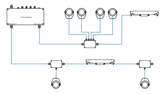
From point of view of driver load (E-box Remote/E-box Remote Basic), max. number of Calummas connected to one E-box Remote/E-box Remote Basic is 40 but Calummas XS have to be operated in the Pass-through mode, it means that max. 32 Calummas XS can be connected in one string.
