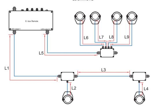
Total cable length=L1+L2+L3+L4+L5+L6+L7+L8+L9
