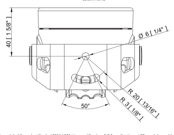
The LED module (4) can be tilted +180°/-180°. Use an Allen key 2.5 for adjusting a LED module position.
