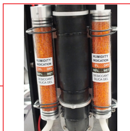
Silica gel desiccants in the fixture arm
