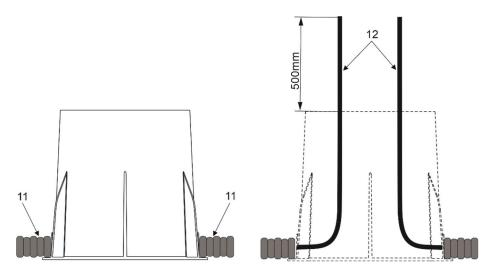
**6.** Fold cables (12) to the mounting sleeve and screw the temporary cover (2) back on the mounting sleeve with three screws (10).
