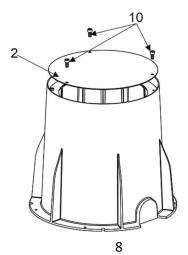
7. The mounting hole can be filled up with soil, gravel or concrete. Filling material should be in the same level with the top of the mounting sleeve (for Bevel Edge Trim) or in the same level with top of mounting sleeve cover (for Flush Trim).
