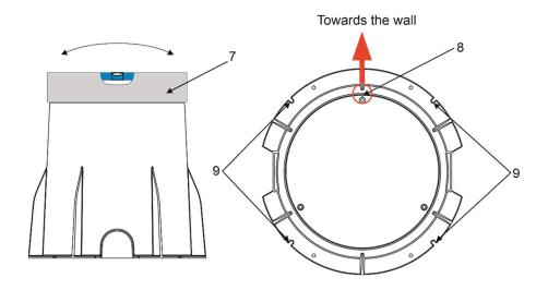
The position mark (8) on the mounting sleeve and the temporary cover serves for orientation of the mounting sleeve and should be oriented to the wall for correct direction of the light beam tilting. The position mark (8) also serves for orientation at placing the Lyrae M to the mounting sleeve. The beam can be tilted towards the teeth (16) in the housing of the Lyrae M.
