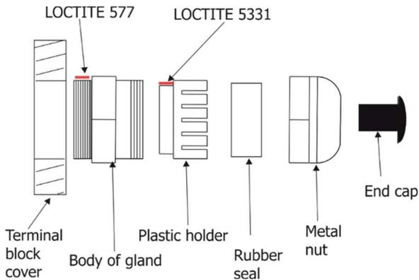
We recommend to apply an adequate layer of the paste LOCTITE 5331 on the plastic holder of the cable gland before inserting it into the body of the gland and an adequate layer of the paste LOCTITE 577 on the thread of the gland body in case that you need to unscrew and remove the cable gland from the housing of the junction box and screw it back to the housing.
