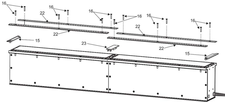
Note: If the Emineres Inground II are installed in a loose soil (e.g. sand, gravel) the cover plate support (25) has to be fastened under the cover plate at outer (end) Eminere Inground II. Screw the cover plate support (25) on the outside of the Eminere Inground II by means of two screws Allen bolts M5x10 with washers and nuts M5.
