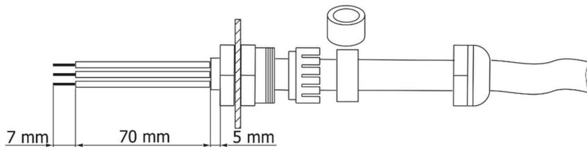
**Reducing seal (P/N 13051388)** - enclosed, standard seal has to be removed before installing this seal
