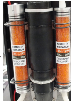
Silica gel desiccants in the fixture arm
