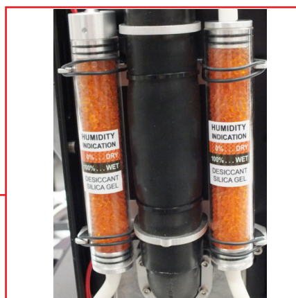
Silica gel desiccants in the fixture arm
